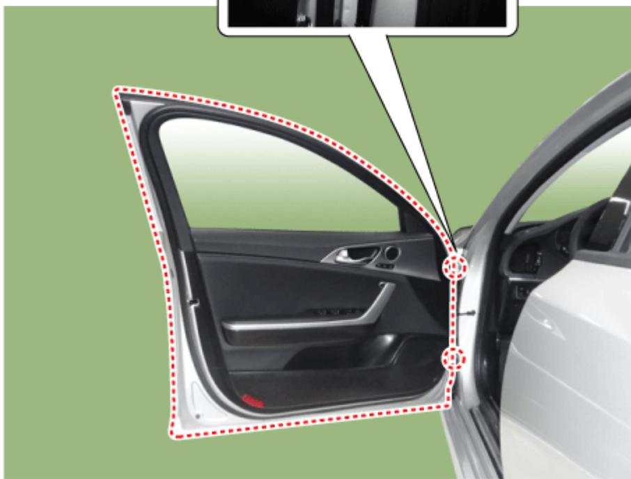
4. Grease the pivot portions of the hinges indicated.
