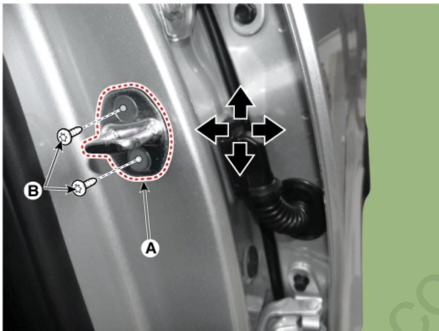
2. Tap on the striker with a plastic hammer to adjust the striker. The striker will not move much, but will give some adjustment.
